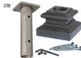
HF16.3.14 Newel mounting kit with level base shoe, fits 1-3/16" round newels, 3-1/8" square base, cast iron
