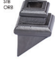
HF16.3.39 Angled base shoe with set screw, fits 5/8" square balusters, 1-1/4" base, cast iron
