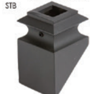
HF34.3.2 Angled base shoe with set screw, fits 3/4" square balusters, 1-7/8" base, aluminum
