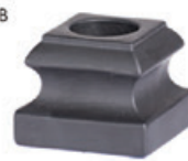
HF16.3.50 Level base shoe with set screw, fits 5/8" round balusters, 1-5/16" square base, aluminum
