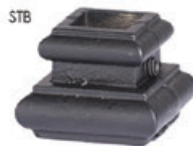
HF16.3.25 Level base shoe with set screw, fits 9/16" Tuscan square balusters, 1-1/4" square base, cast iron
