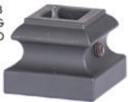
HF16.3.19 Level base shoe with set screw, fits 1/2" square balusters, 1-5/16" square base, aluminum
