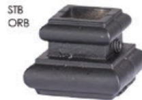
HF16.3.38 Level base shoe with set screw, fits 5/8" square balusters, 1-1/4" square base, cast iron
