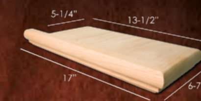
Left & Right Hand Mitered Tread Cap Depth: 13-1/2" Width: 6-7/16" Thickness: 1/2" (1-7/8" Trim) 8071-L 8071-R Red Oak(Ro), Paint Grade(PG)
